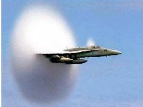
**Figure 1.1: Supersonic F/A18 Hornet aircraft creates a condensation cloud as it accelerates through the sound barrier.**
