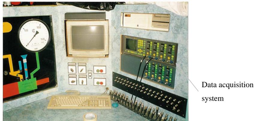
Figure 2.6: Photograph of the data acquisition system of the shock tube
