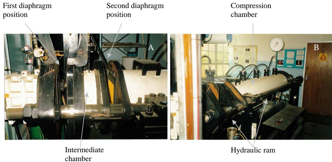
**Figure 2.3: Photographs of driver section of the shock tube.**
