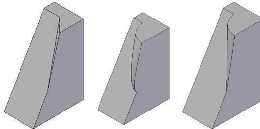
**Figure 2.17: Triangular, parabolic and conical hill test pieces**
