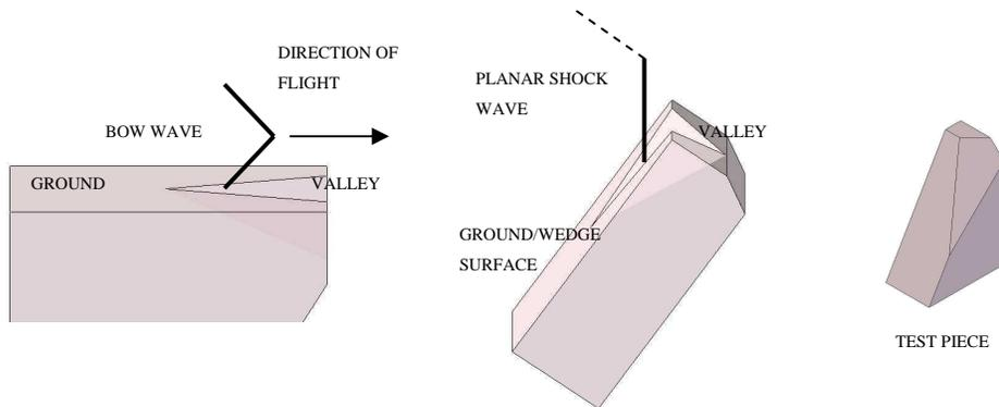
**Figure 2.9: Schematic representation of a supersonic aircraft entering a valley**
