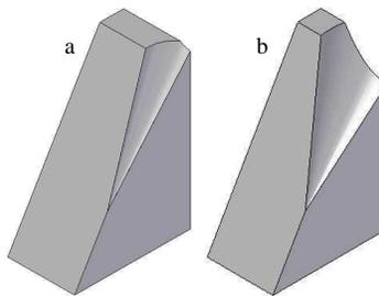
**Figure 2.15: Conical valley test pieces**
