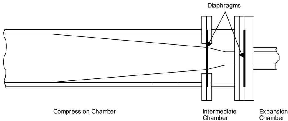
**Figure 2.2: Cross-section of the shock tube illustrating contraction geometry and diaphragms.**
