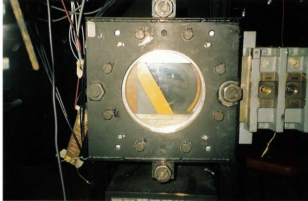
**Figure 2.5: Photograph of test section of the shock tube.**
