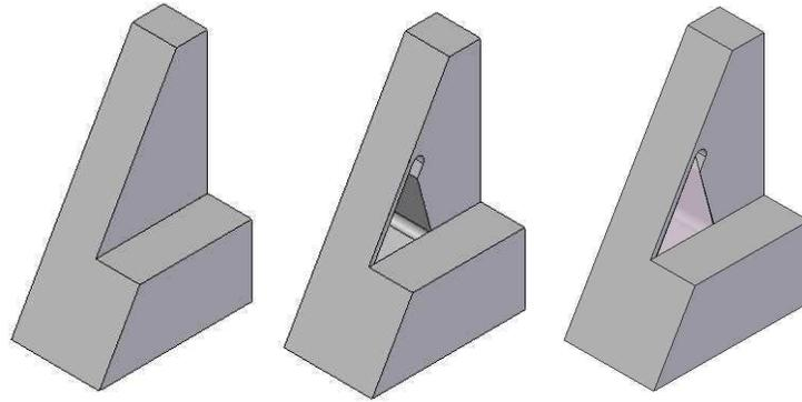
**Figure 2.16: Rectangular valley test piece ( $\theta_w = 60^\circ$ ,  $\theta_v = 0^\circ$ ) with glass insert**
