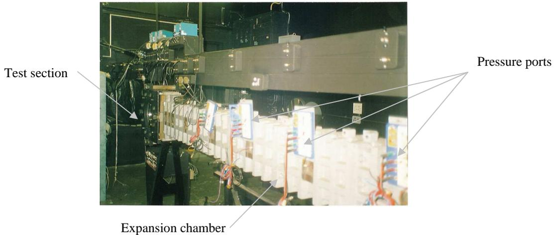
**Figure 2.4: Photograph of expansion chamber of the shock tube.**
