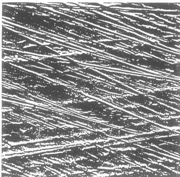
Fig. 3. Enamel surface polished with 600 grit SiC. SEM X 2000.
