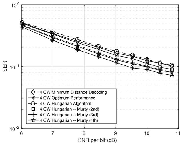
Fig. 3. Performance of soft-decision decoder in AWGN & rayleigh fading channels using 4 codewords (CW).
