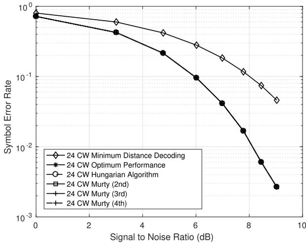
Fig. 2. Performance of soft-decision decoder in AWGN channel using 24 codewords (CW).
