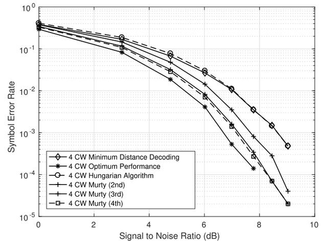
Fig. 1. Performance of soft-decision decoder in AWGN channel using 4 codewords (CW).
