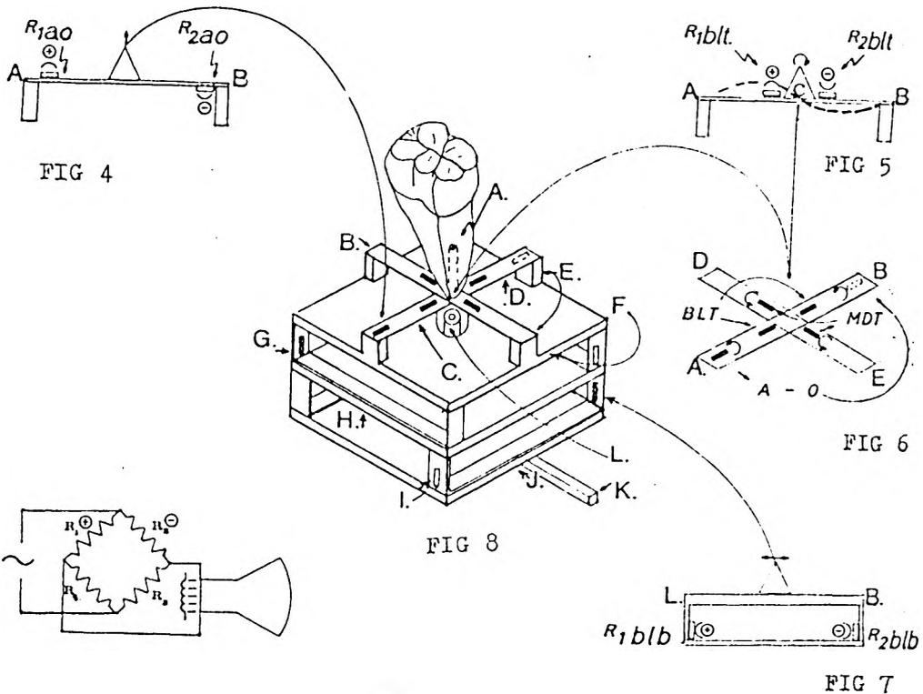
Figs. 4, 5, 6, 7, 8. Design of an omnidirectional transducer.
