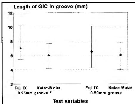
Figure 3: Maximum, minimum and mean values of the length of Fuji IX® and Ketac®-Molar spread within the two groove widths. The comparison within the 0,25 mm groove was significant ( $P<0.05$ ) as indicated by the asterisk, but not the 0,5 mm groove.
