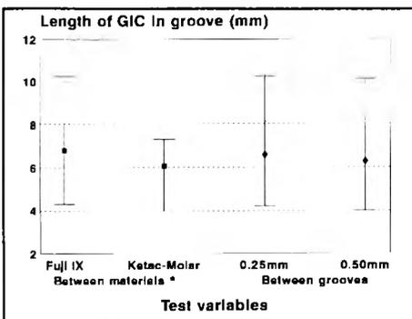
Figure 2: Maximum, minimum and mean values of the length of GIC spread within the grooves. On the left is a comparison between the two materials, which proved to be statistically significant ( $P<0.05$ ) as shown by the asterisk. On the right a comparison between the GIC spread in the two grooves which showed no significance.
