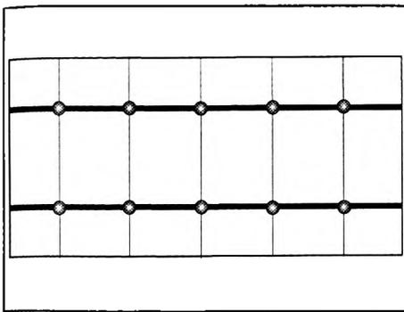
Figure 1: Dimensions of the perspex test mould with grooves and cavities. The heavy line indicates the 0,5 mm groove, the light line the 0,25 mm groove. Cavities are indicated by circles.
